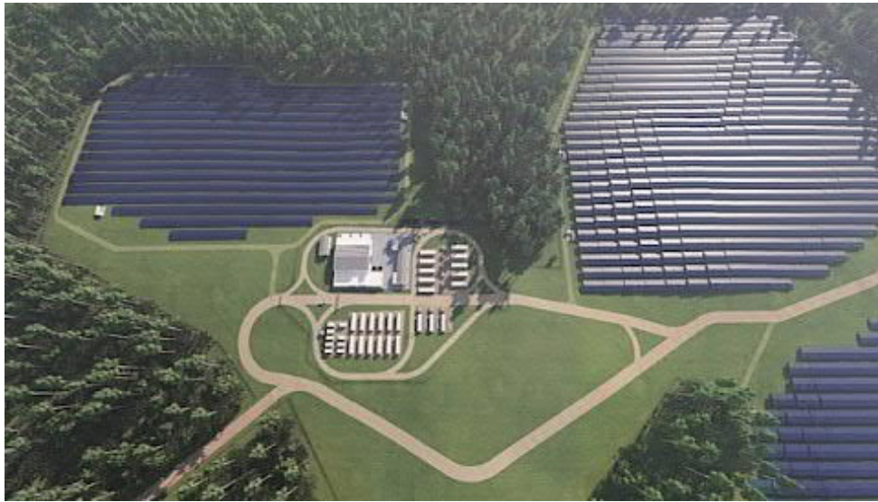
Figure 53: Rendering of 55 MW solar, a 16 MW electrolyzer, storage tanks and 3 MW of fuel cells.
