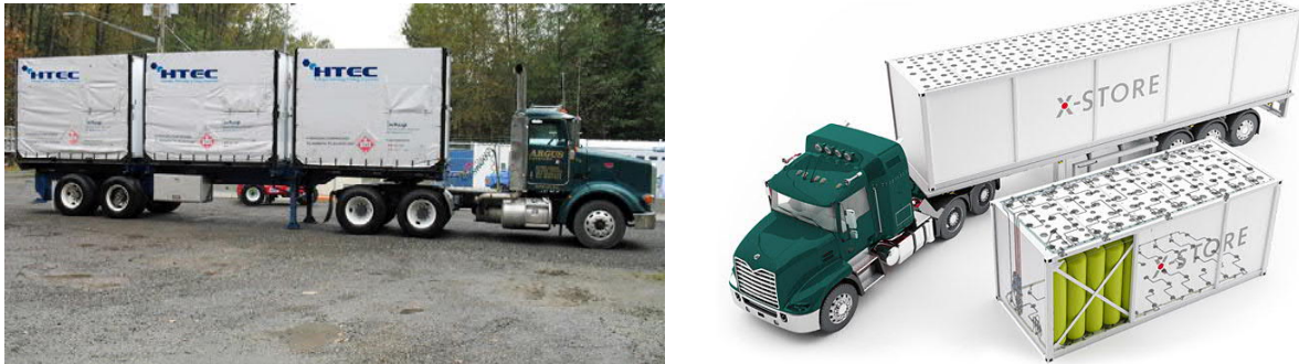
Figure 32: Mobile 450 bar GH 2 Storage Systems from HTEC (left) and Hexagon Purus(right)
