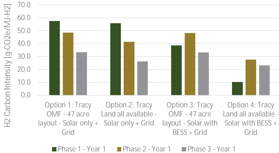
Figure 37: Carbon intensity of the hydrogen dispensed in each onsite hydrogen production project option and each project phase (note: the carbon intensity of the California grid will decrease for future phases)
