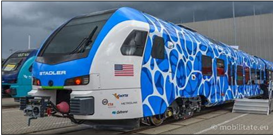
Figure 3 – 2-Car Hydrogen ZEMU Rail Vehicle Developed for Redlands Arrow Project
